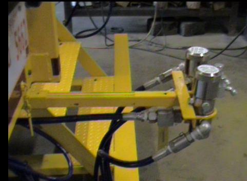
Filters extend from machine to eliminate drips when cleaning.
