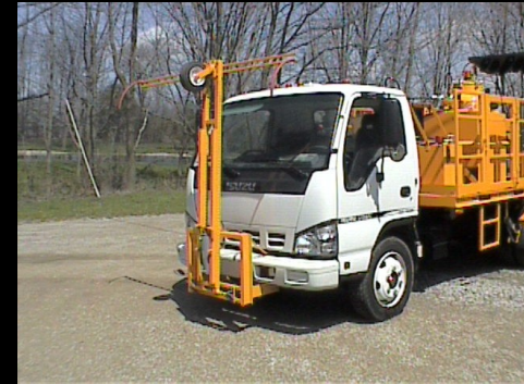
Center-Mounted T-Pointer can touch both edge and center lines simultaneously. Air-actuated pointer lift tilts 45 degrees.
