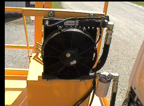
12V oil cooler increases hydraulic efficiency
