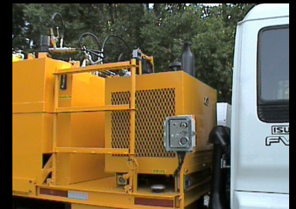
Kubota engine cover with removable side panels for access
