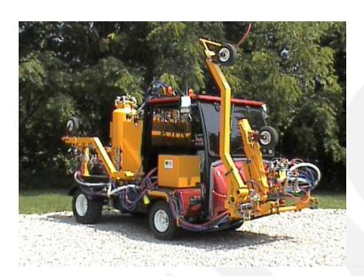
This striper is built on a Toro Workman cab and chassis It has a divided 60-gallon stainless steel paint tank for 30 gallon of each color. It has an edge-line out-rigger and a two-position front centerline out-rigger. All paint equipment is waterborne compatible. An optional set-up for pumping from a 55-gallon drum is available.
