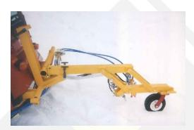
The front centerline carriage is mounted in the middle of the chassis to allow traffic to get around on either side. It has two positions: Extended (left) is for visibility of the paint guns, while Retracted (right) is for tighter radii.
