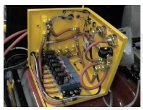
The inside control console has a 3-sided quick-latch removable cover. It houses solenoids and other control components.
